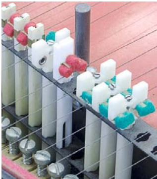
Hubbard jack in center wearing reclaimed Herz damper (red).
