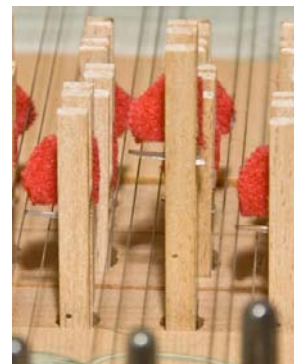
The jack is fully lifted and the string free of damper interference.
