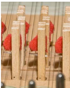
Jacks at rest. The projection of the plectrum past the string can be clearly seen despite the perspective.
