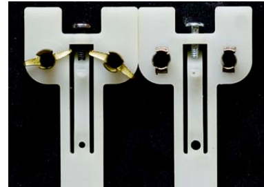
Two Baldwin jacks, dampers removed. Each has lost its integrally molded plectrum. Note the difference in the damper mountings. The jack on the left shows a diagonal orientation (about 30 deg. from horizontal - perhaps derived from the Warner scheme) and that on right, vertical.
