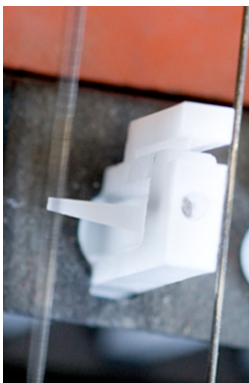
Bass-most string of Baldwin. Right string, still; Left, sounding - note wide excursion. Damper removed for clarity
