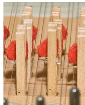
The jack is being let down. On the plectrum's encounter of the string, the tongue escapes backward to allow the plectrum to pass the string.
