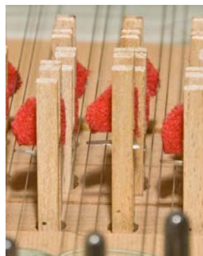
The plectrum of the middle jack has encountered the string. The projection can be clearly seen.
