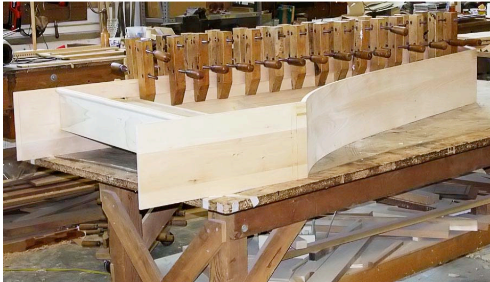
A sturdy bench and lots of clamps ease the task of assembling one of our Flemish kits.
