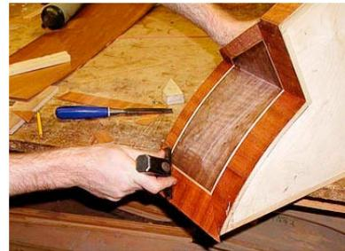
Applying veneer with veneer hammer and hot glue is the traditional method and simple to learn.
